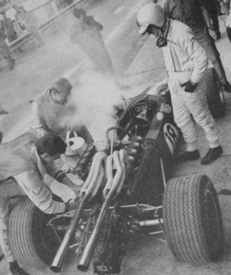
It's a rare GP that Denis Hulme doesn't finish, but at Monza his Repco engine overheated and blew a cylinder head gasket.
