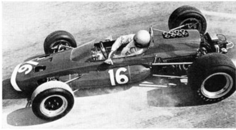
Latest McLaren uses smaller, slimmer chassis with 2.1 BRM V-8.
