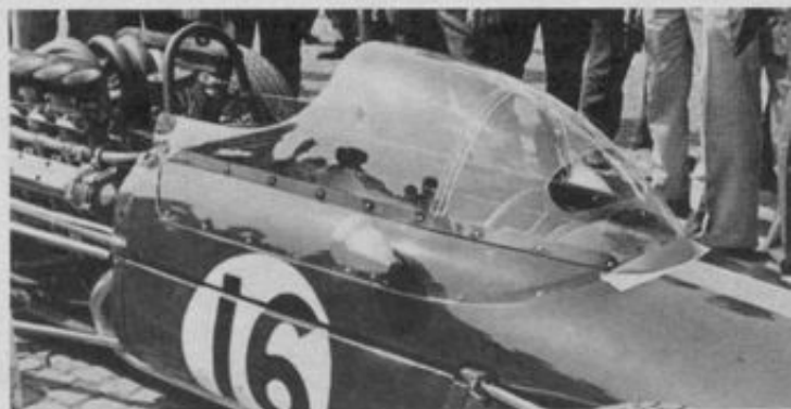
Brabham tried a streamlined plastic cockpit canopy in practice. It gave no extra speed and was not used in the race.
